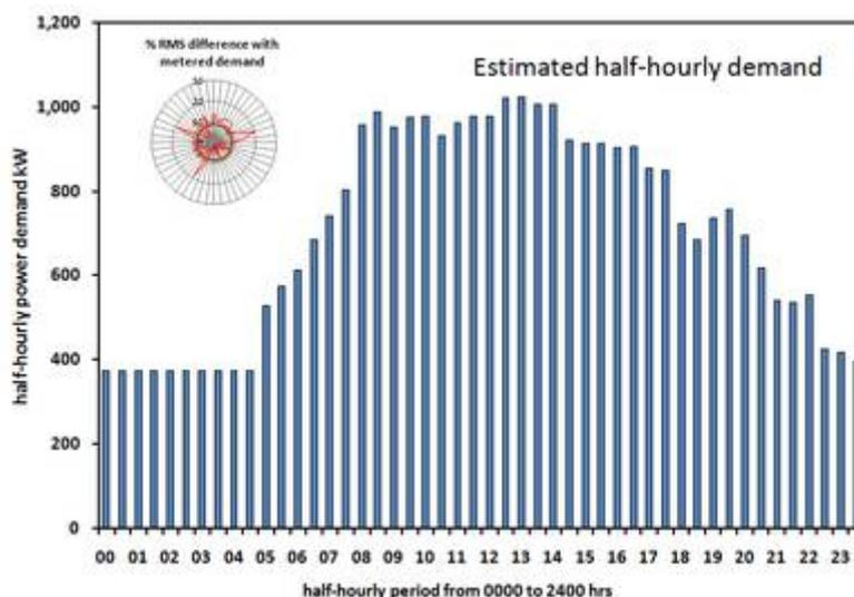
The simulated half-hourly electricity demand over a 24-hour period is shown opposite. The demand profile has been matched to the site. For the 24 hour period, the total simulated electricity demand was 16.9 MWh. The corresponding metered value was 17.0 MWh. Once matched, the simulated profile can be investigated in detail for energy and cost saving opportunities. The inset shows the % rms difference between metered and estimated demand; average over the 24-hour profile is 8%.
